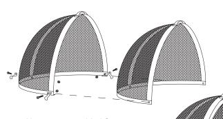
1. Nest two assembled Screen Sections (A) so the welded handles are on top and the hinge sections of both sections are aligned. Attach screens at each hinge by inserting Bolt (E) through a Screen Fastener Clamp and aligned Screen Sections. Loosely secure Bolt (E) with Nut (F). Hand tighten hardware only. Repeat step 2 for opposite hinge. Attach remaining Screen Fastener Clamp (G) with Bolt (E) and Nut (F). Once all hardware is in place, tighten Bolts with Hex Wrench (H).
